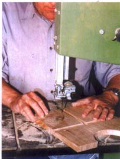
Cutting the front curved edge. Note the first step and panel rebates
