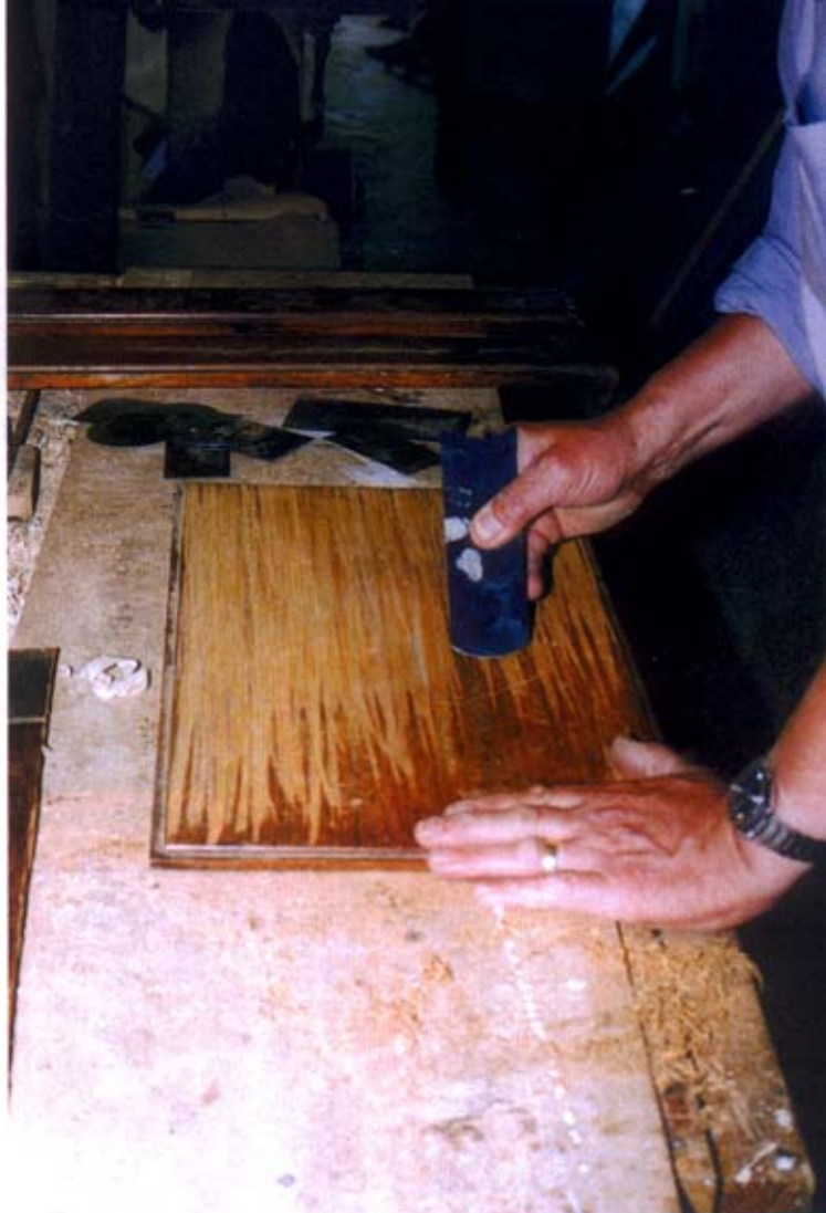
One of the two recycled pieces varnish being dry scraped
