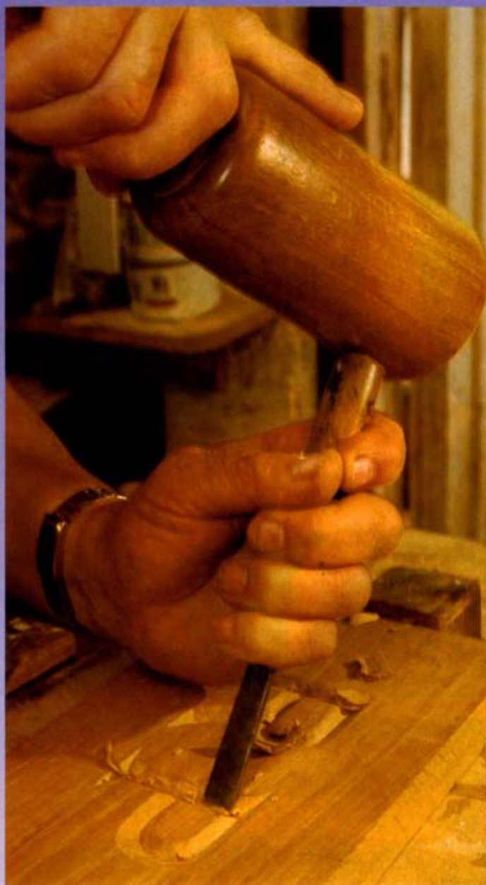
The curved lines are dealt with in a similar manner but with a shallow curved gouge as near to the curve as possible, letters such as an R, B or a P are a little more difficult owing to the tight curves
