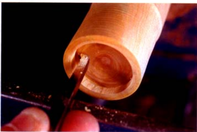
Cut the gap at the end of the thread run
