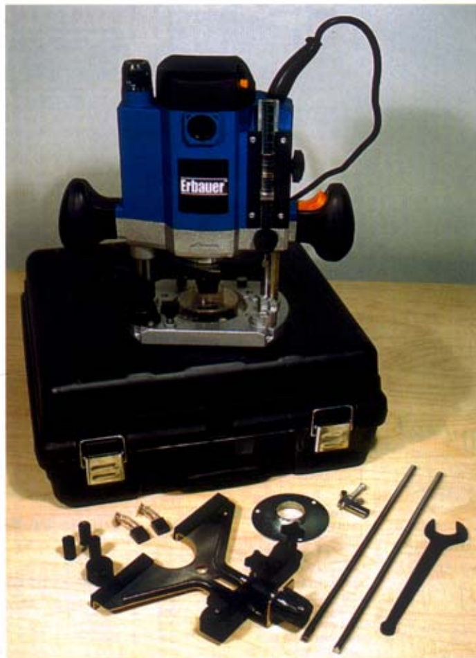
Plunge depth controls and handle incorporating power switch
