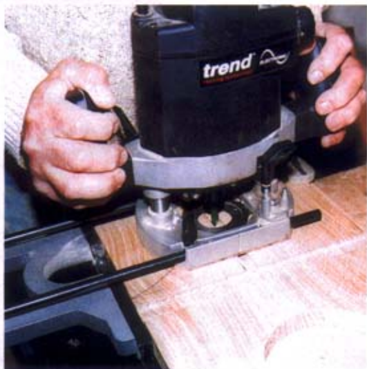
Routing the front panel rebates
