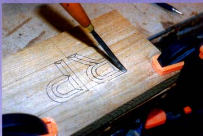
Defining the cut of the angles into the corners from the centre line
