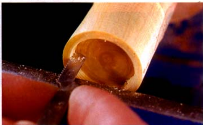
...lift the the thread chaser out of the thread
