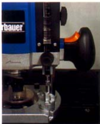
Plunge depth controls and handle incorporating power switch
