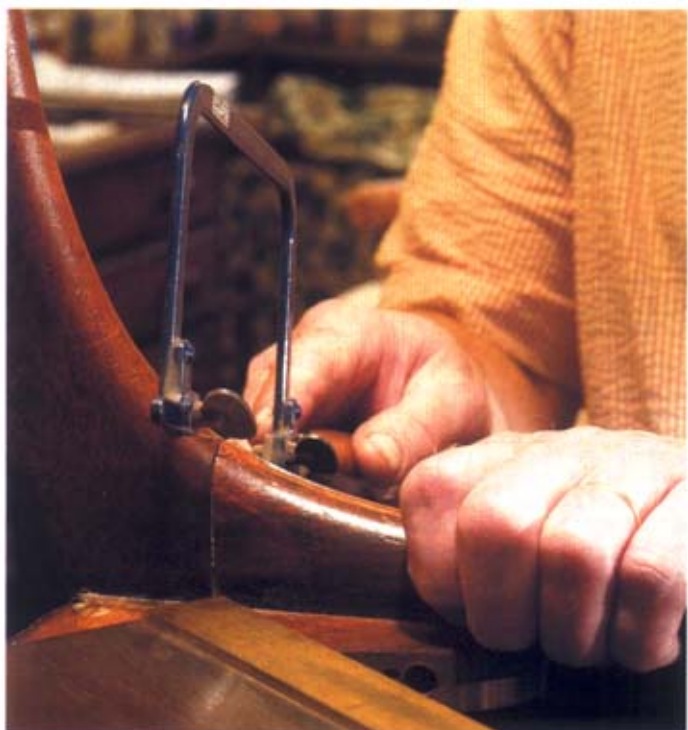
If you have to cut a joint apart make sure you have a fine blade to minimise damage and wood loss. Here you can even use a razor saw or jeweller's blade but never a tenon saw
