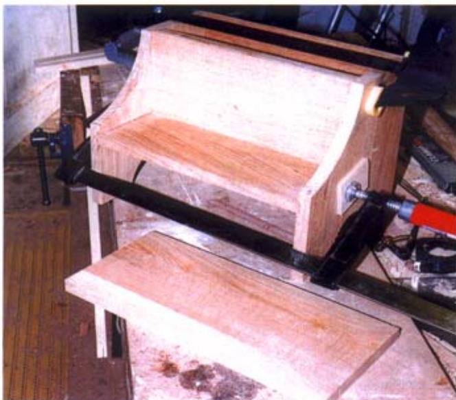
LEFT - Yes, another dry assembly after cutting the front curved edges
