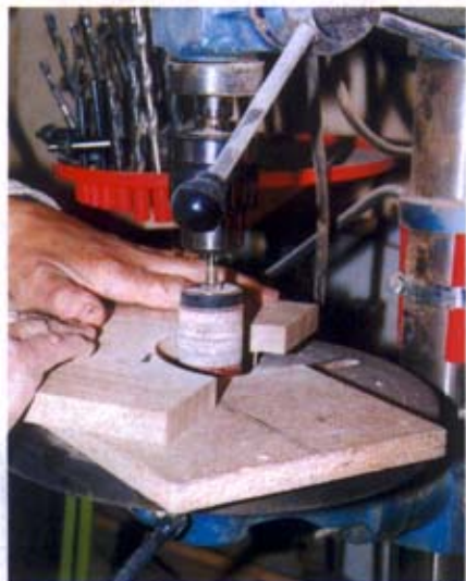
Giving one of the four curves a sanded finish
