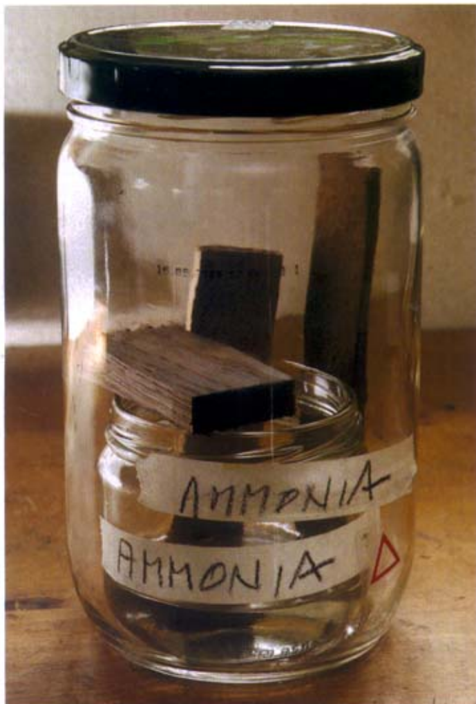
Always be able to see what you are doing. The colour can change quickly and permanently with fuming
