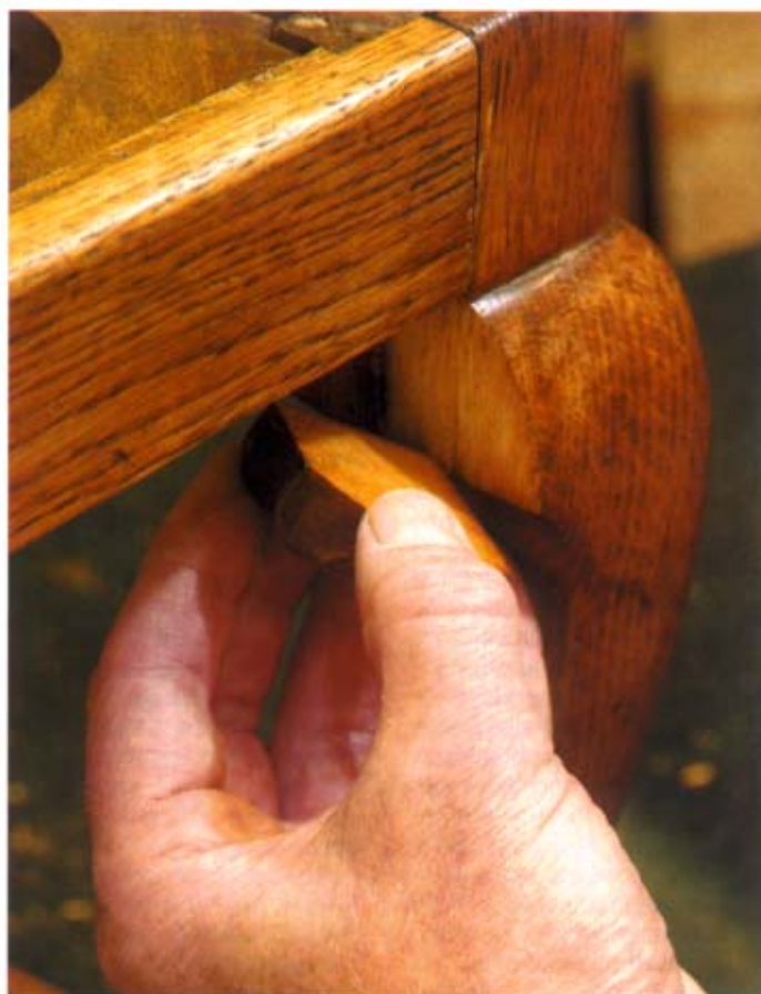
Some mistakes are easy to repair with a simple rub joint...
