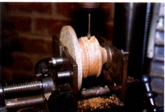
Drilling the hub
