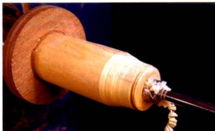
Bore out the hole which houses the mechanism
