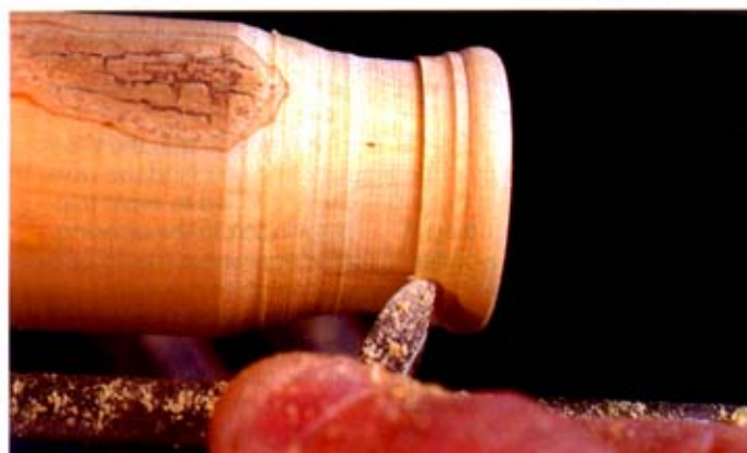
Form the moulding on the side of the lid
