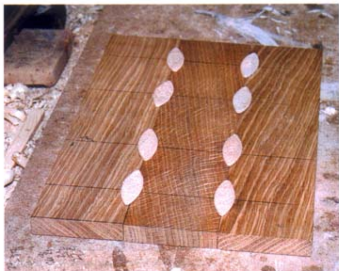
Working out how many biscuits for the first step
